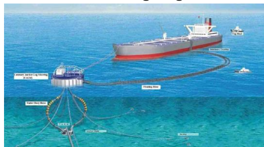
Figure 15: Single Point Mooring (SPM) with Double Pipeline
